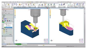
function enables the recognition of 3D shape in CAM. To add to the conventional functions that includes drilling and 2 axis pocket machining, it has brought us to the realization that the practice creates machining data mixed with 3-axis paths in a short time, which is supposed to be difficult for recognizing in 2D shape. The function fulfills the great precision and efficiency in machining since it equips the same operation employed in CAM-TOOL, which has a proven track record in 3 axis paths.
