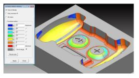
Moreover, 39 functions have been enhanced, including improvement of shading ("Curvature Radius/Angle Shading" in gradation of 7 colors: Picture on the left), functional enhancement of "Surface Plus", strengthening and improvement of toolpaths for machining, extension of usable cutting-tool shapes, and expansion of "Simulations"/ "Tooling DB"/"Translators".
